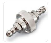
The G<sup>1</sup>/<sub>4</sub> connection threads with density barrel, guarantee leak-proof sealing of the hose nipple and the holder without sealing rings. Other connectors, available as accessories, fit the holder onto reducing valves or pumps with G1/4 female thread (order no. 01030) or G3/8 female thread order no. 01029) or onto pressure tanks with G3/8 male thread (order no. 00177).
