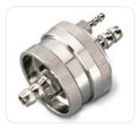
The filter holder is suitable for a pressure of up to 20 bar. The inletside valve is convenient for the intermittent run-off of waste water. Other connectors, available as accessories, fit the holder onto reducing valves or pumps with  $G_{3/8}$  female thread (order no. 17089) or onto pressure tanks with  $G_{3/8}$  male thread (order no. 17069) or on taps with  $G_{3/4}$  male thread (order no. 17068).
