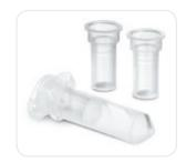
Vivaclear centrifugal filters are disposable microfiltration devices for the fast and reliable clarification | filtration of biological samples in the range 100  $\mu$ l to 500  $\mu$ l. They can be used in fixed angle rotors accepting 2.2 ml centrifuge tubes.
