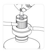
To fill multiple receiving bottles, break the vacuum with the valve on top of the Sartolab<sup>®</sup> 150v housing.
