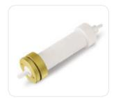
The holder hinders the release trace elements into the filtrate and is resistant to almost all chemicals. The Viton O-ring in the top part allows easy hand tightening, and can be replaced by a PTFE O-ring, order no. 17039. The 6 mm outlet nipple is an integral part of the base, the 10 mm inlet hose nipple can be replaced by a G<sup>3</sup>/<sub>8</sub> connector, order no. 17051.
