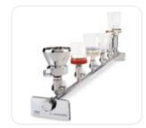
Made of high-grade stainless steel (B.S. 304S3 | AISI 304); accommodates any type of vacuum funnel. Stainless steel three-way valves (taps) allow the vacuum for each filter holder to be individually controlled and each holder to be sterilely vented. The low height of the manifold ports is particularly advantageous for working on a clean bench.
