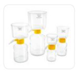
Sartolab<sup>®</sup> Disposable Sterile Filter Systems and Bottle Top Filters are designed for the vacuum filtration of tissue culture media and components, biological fluids, and other aqueous solutions.
